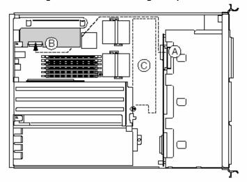
Figure 33: Connecting to a half Height PCI SCSI Controller
